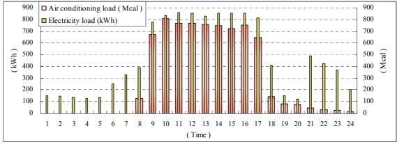
Figure 5 Electricity load and an air conditioning load pattern of one day
